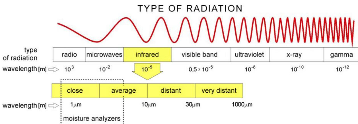
Fig. 2. Division of electromagnetic waves
