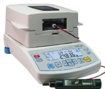
It is important to remember that both thermometers (integral part of moisture analyzer, and test thermometer) should be equipped with probes of the same colour. In case where one probe is light (stainless steel), and the other is dark, there may occur errors sourcing from:
